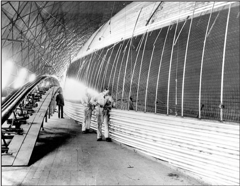
Slate Aircraft Co. Workers assemble the aluminum hull of the City of Glendale.
