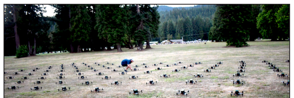
A fleet of 140 Verge Aero drones went through pre-flight structural checks along with GPS confirmations to ensure they would maintain precisely aligned positions, linked with each other.
