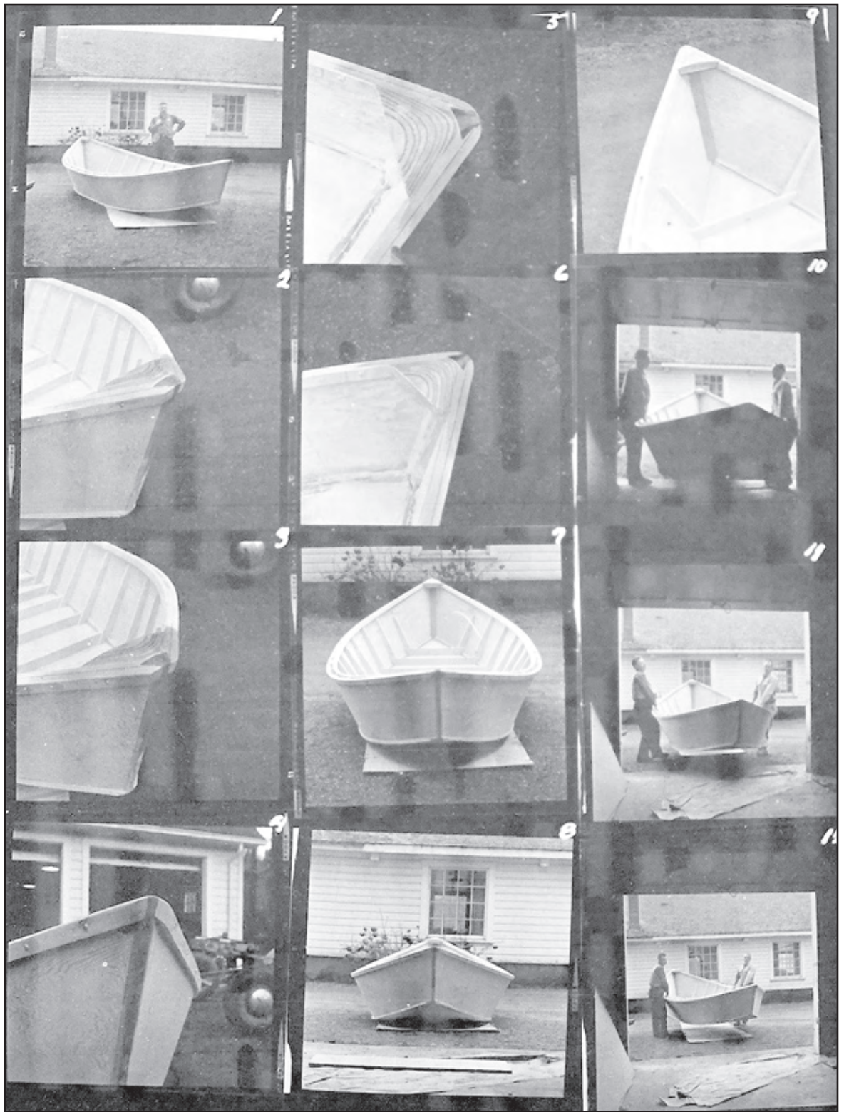
Six inches wider than a traditional McKenzie boat, the Colorado boat constructed at the Old Leaburg Hatchery in 1962 had a flat midsection to help it float a bit higher, combined with curved rocker ends for maneuverability while pivoting.
