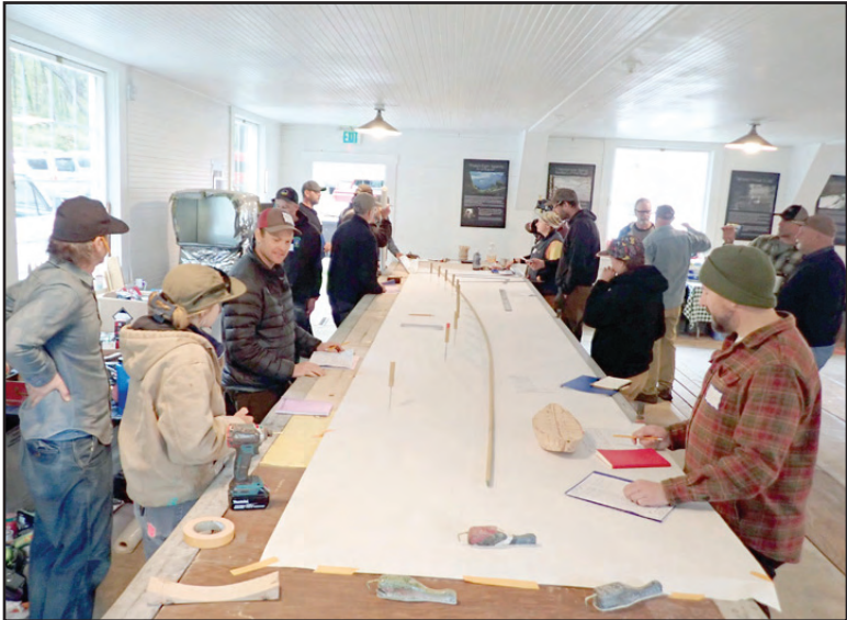
Learning how to loft the boat from a set of offset numbers on Day One.
